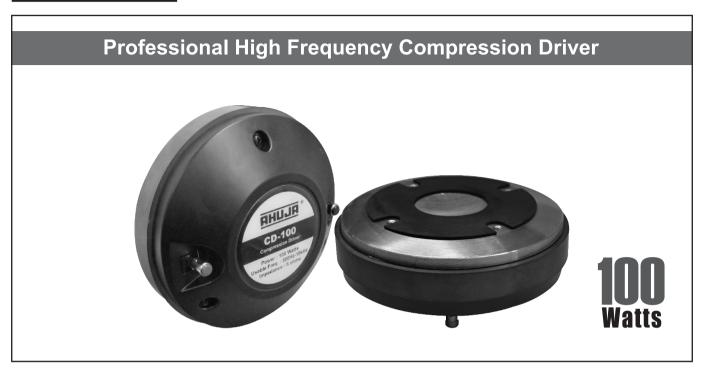
Ahuja introduces a 100W, 2" throat compression driver model CD-100, suitable for use with high power LF speaker systems. It features Titanium diaphragm and Aluminium Ribbon Wire voice coil for delivering loud and crisp Mid & High frequency response. Suitable for use with HF horn similar to Ahuja model H-7380.
