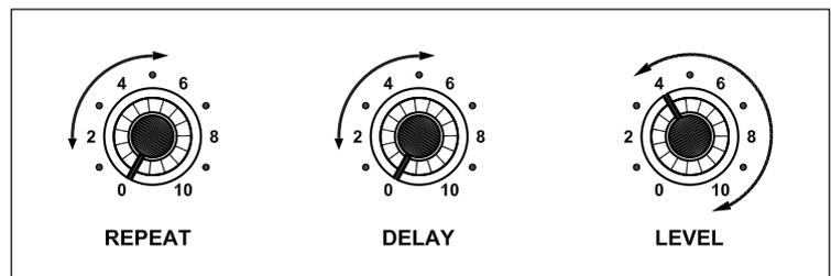
**CHORUS** - Chorus Effect is used by a singer to create an effect as if a Group is performing. The control settings for Chorus are as shown in the diag.
