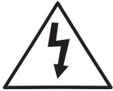
This symbol, wherever it appears, alerts you to the presence of uninsulated dangerous voltage inside the enclosure, that may be sufficient to constitute a risk of shock.
