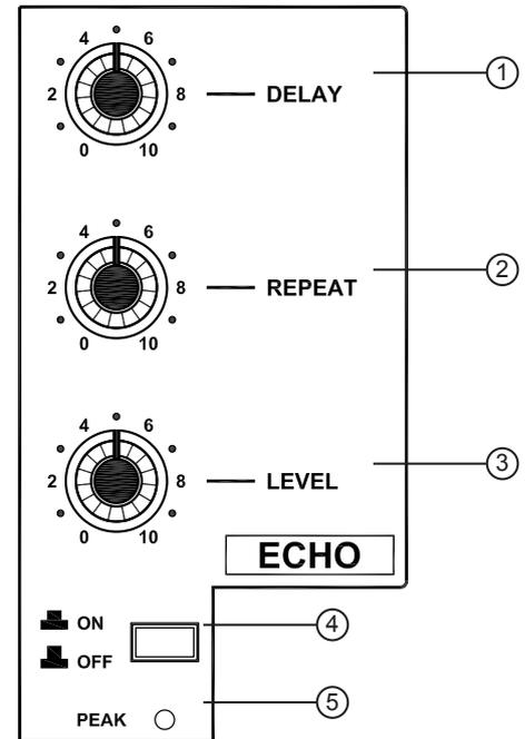
**ECHO** - Echo Effect is used to repeat the original sound many times to give multiple voice effect and is used for vocals. The Control settings for Echo are as shown in the diag.
